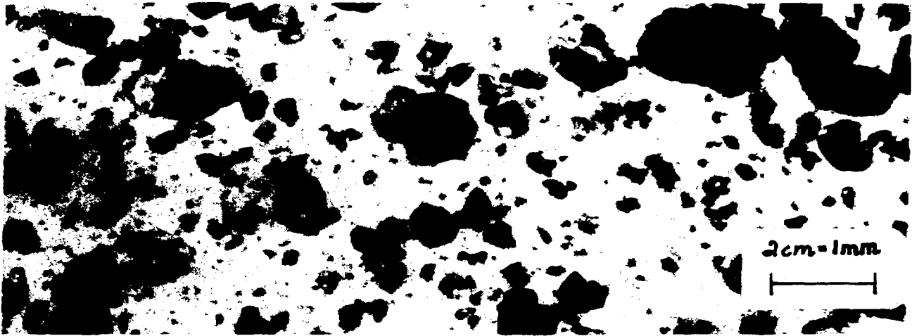
Figure 6.2 Micrograph of a cross section of polyethylene/ \text{NaNO}_3 (50 wt%) waste form.
