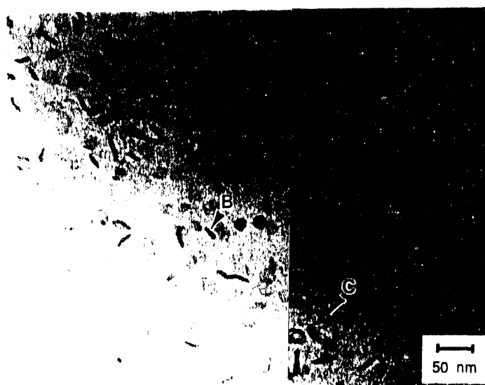
Figure 7. DPPC and DHPC mixtures at 45° show discoid structures. The discs appear to be oblate spheroids and are seen in various orientations with respect to the electron beam: (A) Axis of revolution parallel to beam gives circular image 20-30 nm in diameter, (B) Axis of revolution perpendicular to beam gives line 5-6 nm in diameter, and (C) Axis of revolution at other angles gives elliptical shapes.
