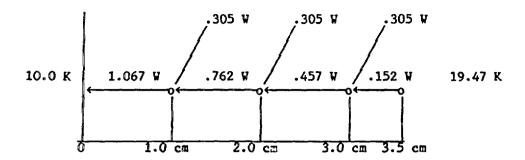
The calculation indicates the with a 6 % density, 10 PPI, 6101-T6 Duocel foam metal a maximum temperature of 19.47 K can be expected at the hottest point in the moderator. The moderator actually operates with the full heat load and with helium gas at 7 K, at a temperature of 12 K in the location of the thermocouple.
