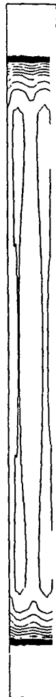
Figure 12. Simulated interferogram for the diffuse reflector with 48°C end coolant temperature. One slab thickness has been removed from each end. The contour interval is 1/2 wave.
