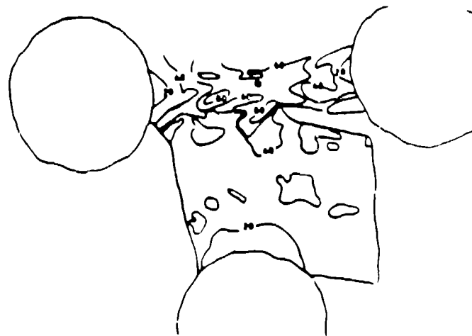
Figure 4. Experimental Von Mises strain distribution
