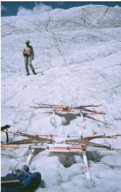
Photo 4: Ground penetrating radar antennas.
