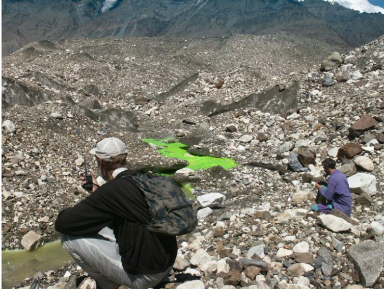
Photo 5: Colored meltwater after the injection of the tracer.
