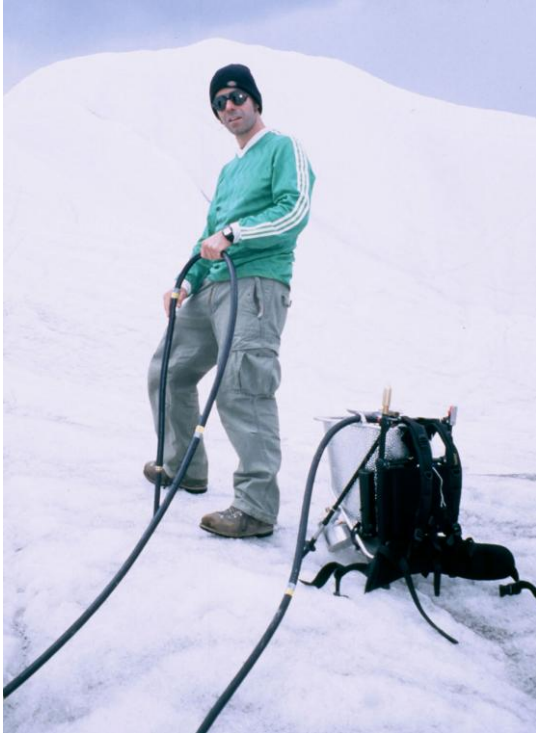
Photo 2: The Heucke ice drill is able to penetrate glacier ice up to 15 m depth.
