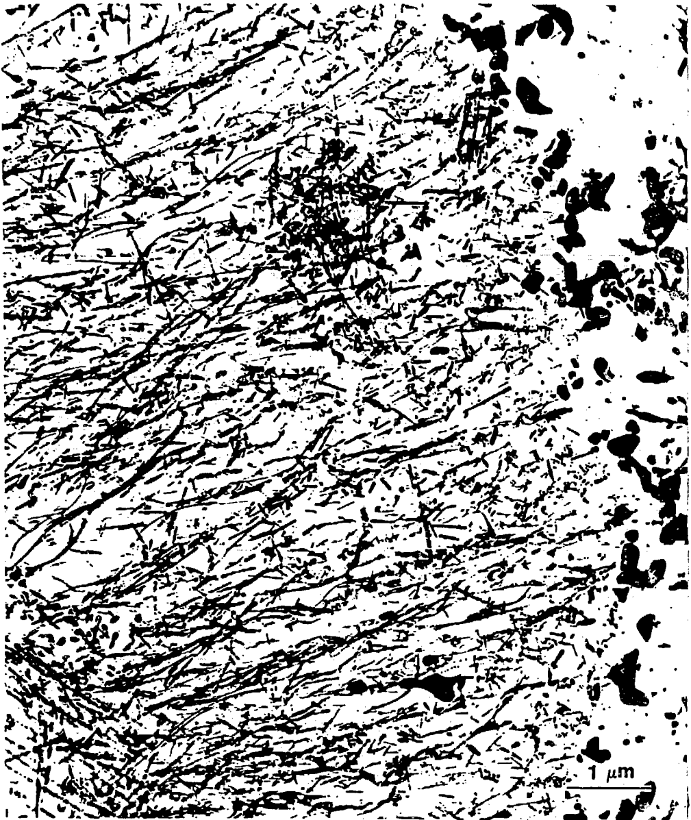
Fig. 5. Extraction replica that shows an example of coarser fiber or "ribbon" precipitates that occur in the polygonal ferrite of the normalized-and-tempered 2%CrV.
