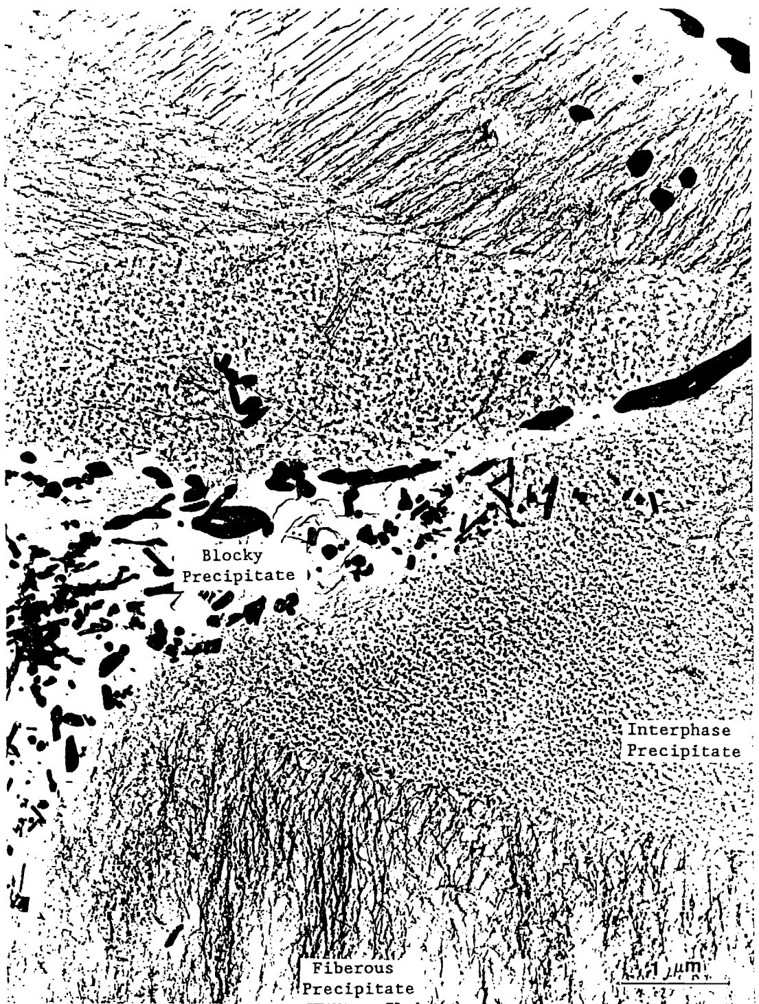
Fig. 4. Extraction replica that shows an example of the fibrous, interphase, and blocky precipitates that occur in the polygonal ferrite of the normalized-and-tempered 2%CrV.
