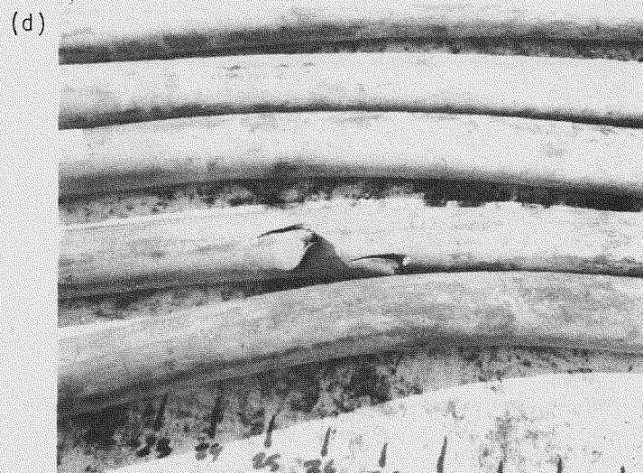
Figure 12. Sections from the bottom part of the polar crane pendant: (a) Cables 16-8. (b) Reverse sides of cables in (a). (c) Lengths 3-5, showing insulation cuts and checks. (d) Lengths 8-9, showing charred cut.
