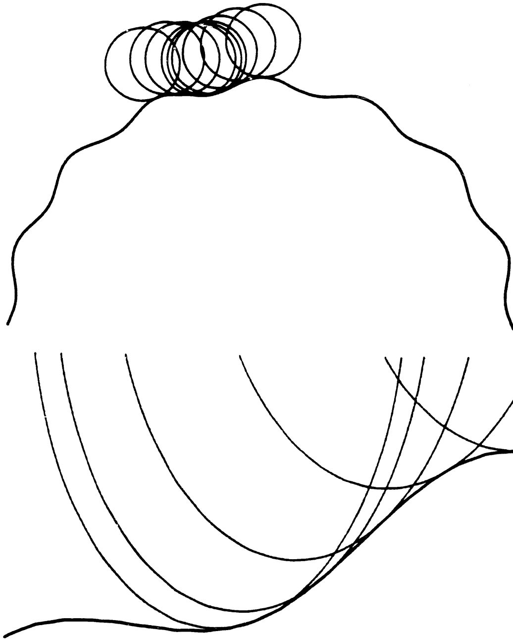
Fig. 17. a) Diagram showing a cross-section of the helical multifoil mode converter with "tool-cut" circles for the case of 8 cuts per period. b) Expanded view of one period of the top drawing with the vertical dimension expanded much more than the horizontal.
