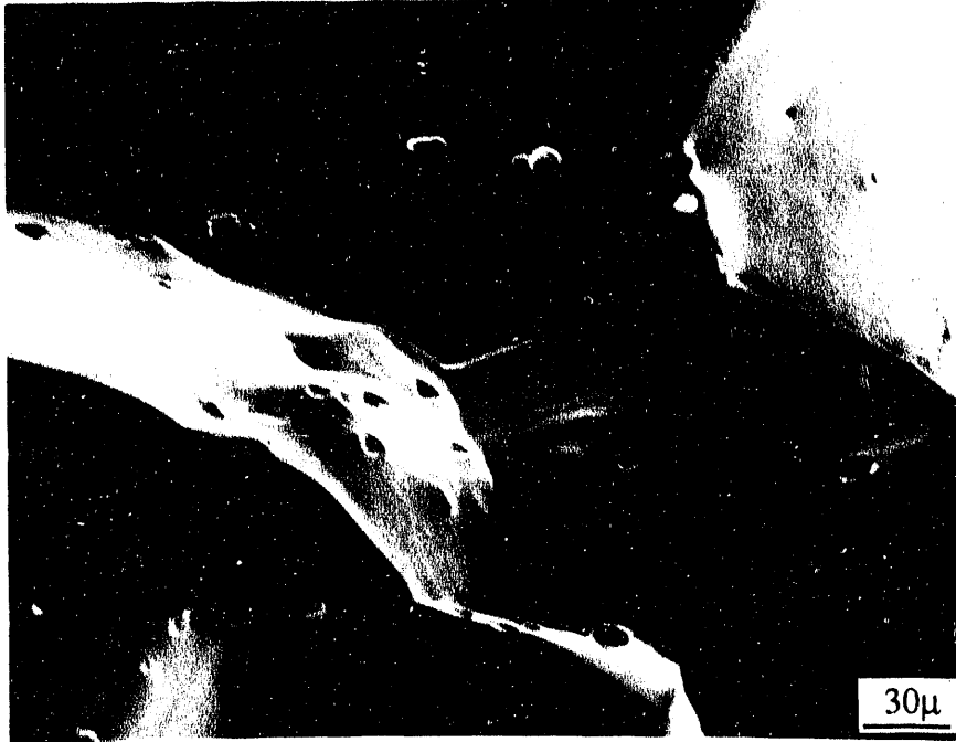
Figure 11. Fracture surface morphology of Inconel 617 hot ductility sample tested for on-cooling at 1127°C.
