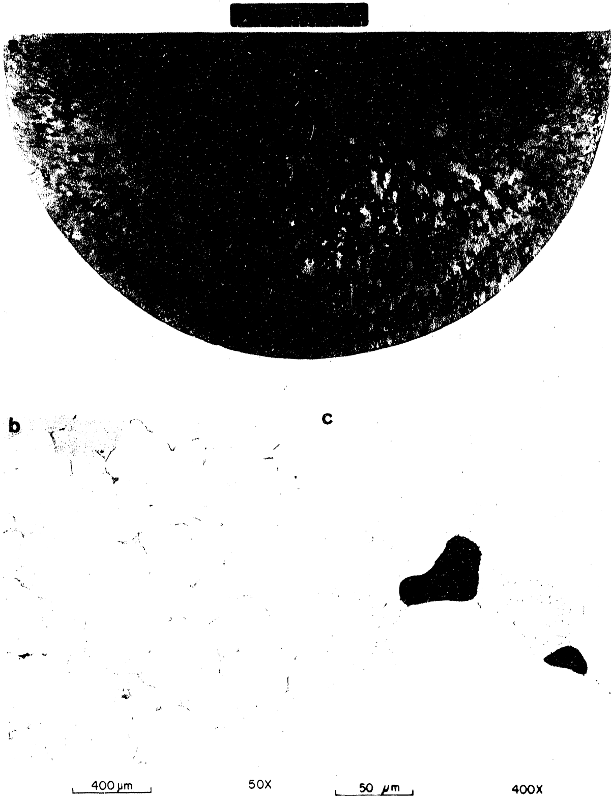
Fig. 7. Optical macrostructure (a) and microstructures (b,c) of a section taken from near the top of the 406-mm-diam ESR ingot of FA-129 showing (b) grain size and second-phase distribution at low magnification, and (c) eutectic and porosity at high magnification.
