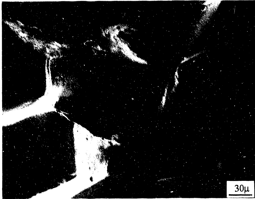
Figure 9. Fracture surface morphology of Inconel 617 hot ductility sample tested for on-heating at 1204°C.
