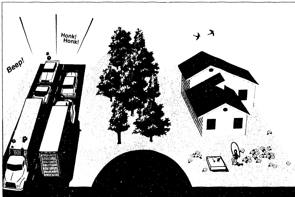
Figure 2-11. Benefits of berm: A row of trees can be particularly effective in screening undesirable urban noise.
