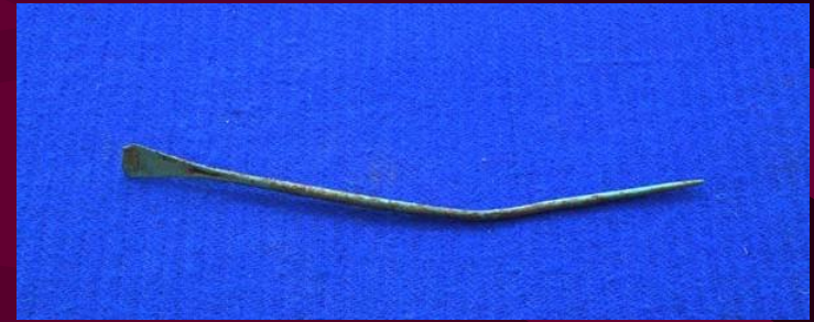
Cold-worked copper needle
