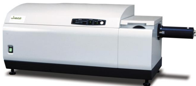
Figure 3. A representative CD spectrometer. The cylinder at right is the detector.
