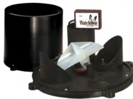
Figure 9.4 Example of an automated rain gauge (Source: Spectrum Technologies Inc.)
