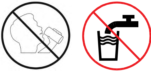
Figure 10.8 Pictographs for (a) DO NOT DRINK [IGCC 706.2] and (b) DO NOT DRINK THE WATER [TAC210.25 (b) (1), GPMCS§503.9]
