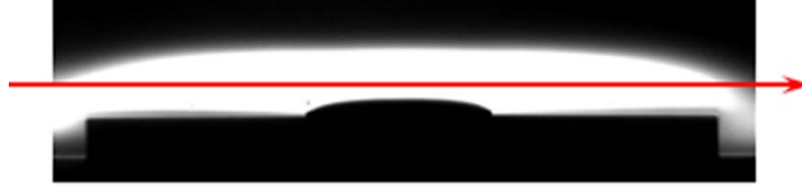
Figure 1. Schlieren image of the vapor cloud surrounding a pinned, sessile hexane drop. The bright region indicates the presence of vapor and the arrow demonstrates a path of the infrared beam from the FTIR through the vapor cloud.
