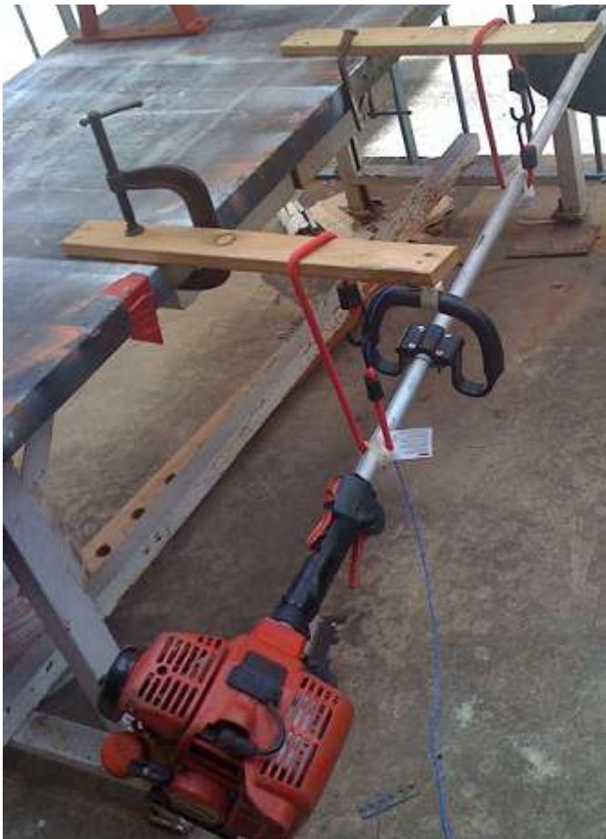
Fig. 5 Free-free suspension approach for string trimmer baseline test. The Shindaiwa trimmer is shown here.
