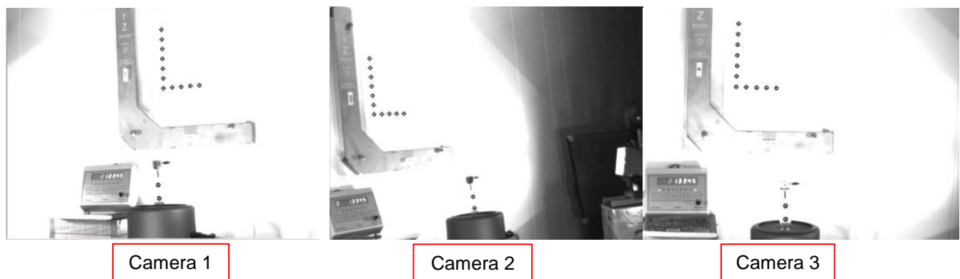
Fig. 5: Once set of the experimental images (epoch) used to calculate acceleration of a sinusoidally-driven shaker. In this experiment, the oscillating shaft was aligned with the horizontal (y) axis of the pictured coordinate axes.
