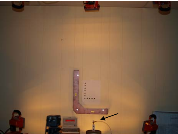
Fig. 3: Uniform, shadow-free illumination of a test object (accelerometer and shaft mounted on mechanical shaker, demarcated by arrow) was accomplished by using an array of eight (five visible) distributed halogen worklights, including one located directly behind the shaker. The upper set of lights was clamped directly to the ceiling tile grid.
