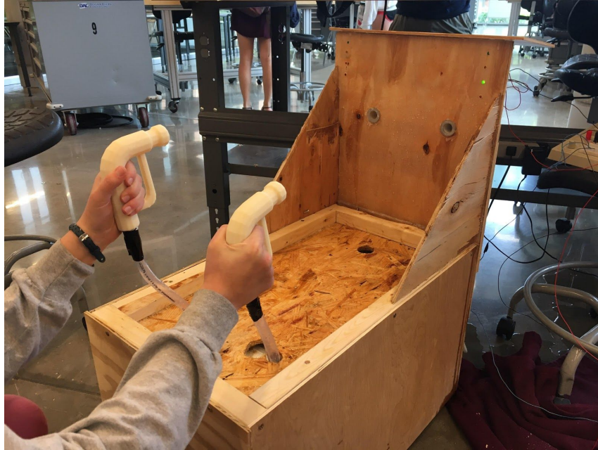
Figure 3: Front view: 3D-printed water guns are connected to a pump that is hidden under the wood casing in an ice chest full of water. There is a target and LED progress bar for each player. The drain at the far end of the tank is used to collect the water that does not go into the targets.
