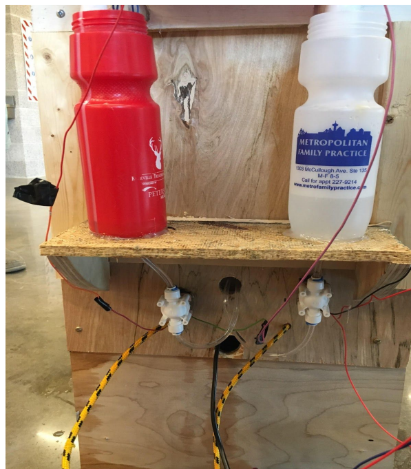
Figure 4. Back view: water bottles collect the water that the users shoot into the targets. The water level sensor wires are fixed at five specific heights in each bottle.
