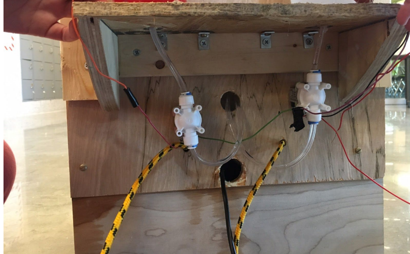
Figure 5. Solenoid valves drain the tanks automatically at the end of each game.. A single exit for the pump wall plug is shown at the bottom. The yellow rope is one of two handles that make transporting the cabinet safe and easy.
