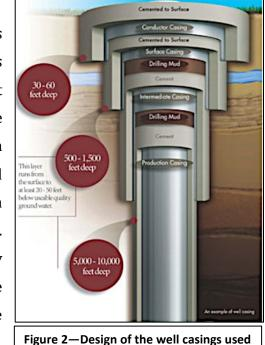
Figure 2—Design of the well casings user to protect aquifers Source: FracFocus
