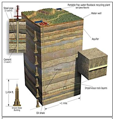
**Figure 1—Diagram of the process of hydraulic fracturing** *Source: FracFocus*
