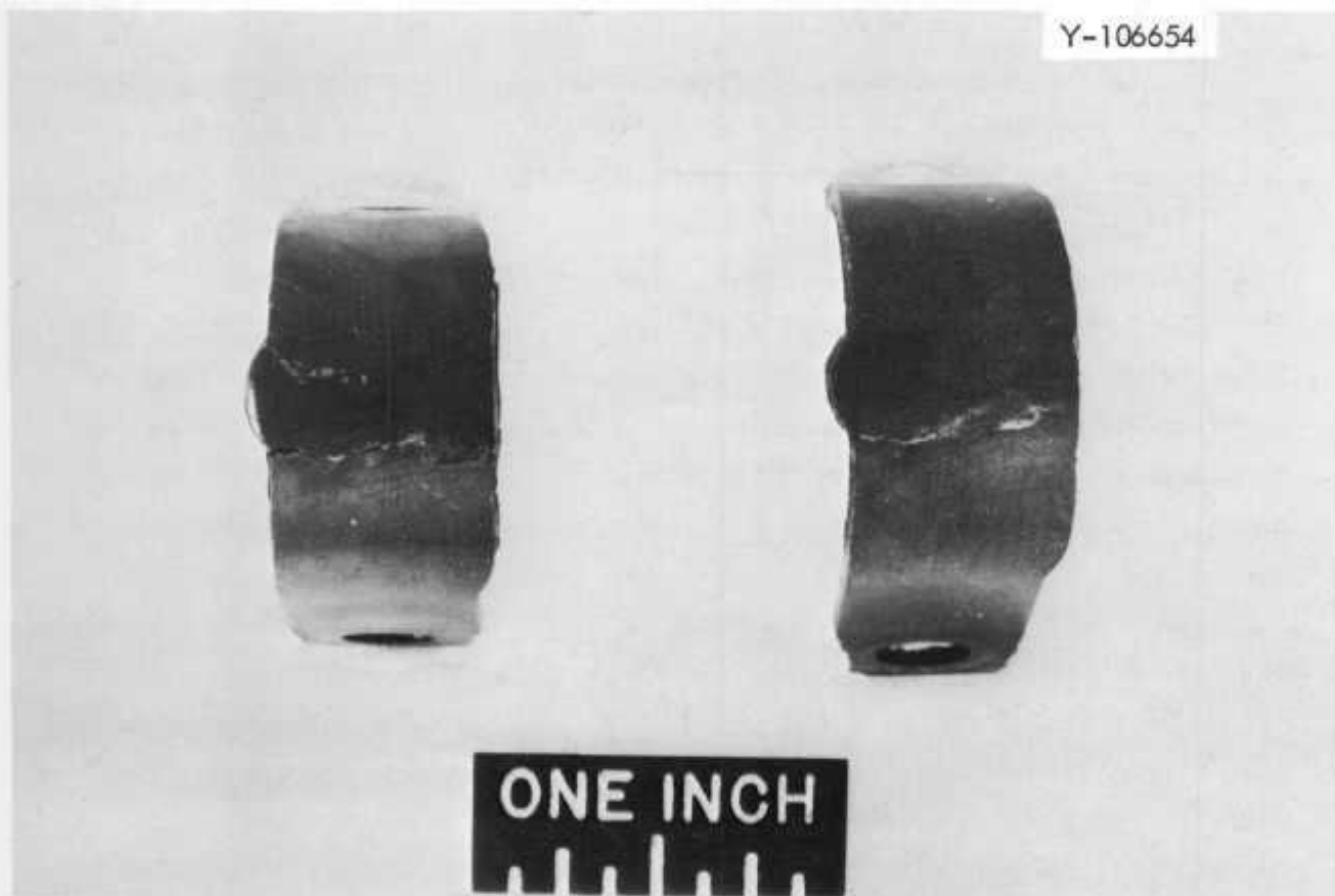
Fig. 20.3. As-Ground U-Bend Specimens of Hastelloy X Welded to Itself (Weld A5), Cracked by Stress Corrosion in NaCl-Contaminated Steam. Cracks initiate at surface adjacent to root pass and progress into base metal alongside fusion line before proceeding into the weld deposit.
