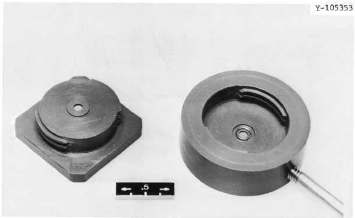
Fig. 3.10. Twist-lock Specimen Holder for Electropolishing. The specimen fits in the recessed area.
