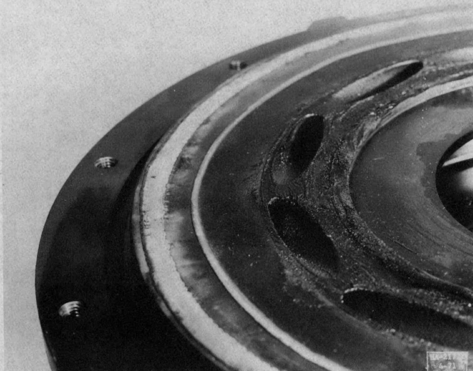
Figure 34 Nozzles Numbers 1 and 2 After Testing
