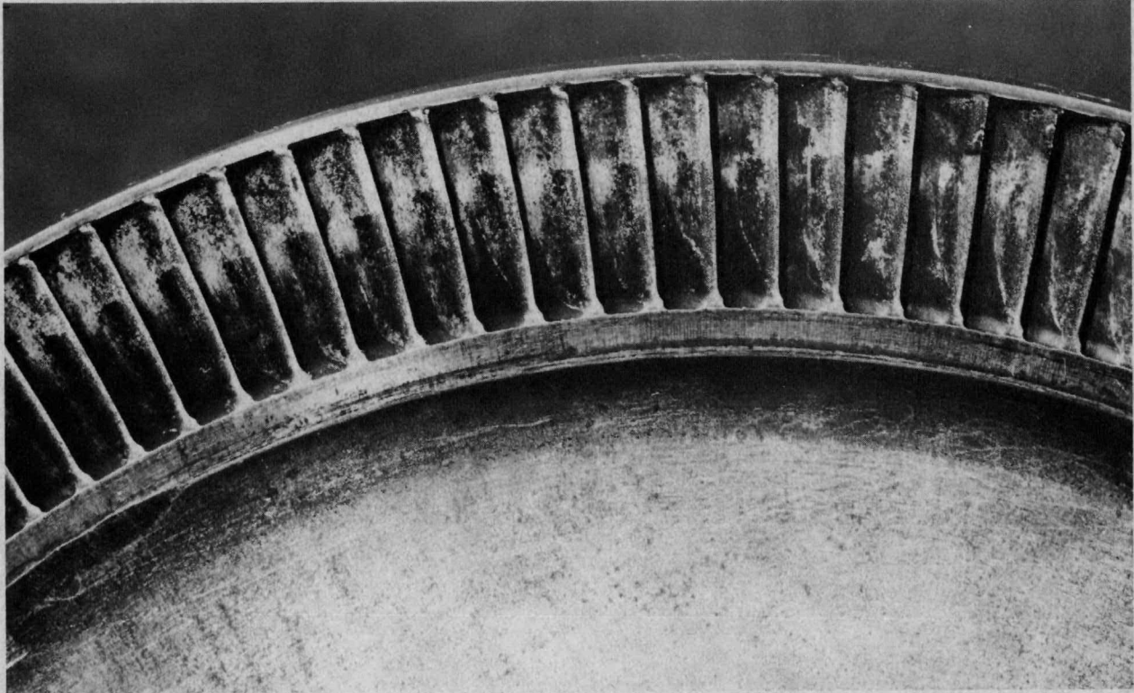
Figure 28 Turbine Buckets After Test (Exit Side)
