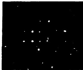
Fig. 1. A self-focusing pattern photographed at the exit face of a CS_2 cell. This pattern originates because of the rapid growth of a spatial perturbation whose k -vector components, k_x and k_y , can be determined by measuring the spacings between the focal spots.
