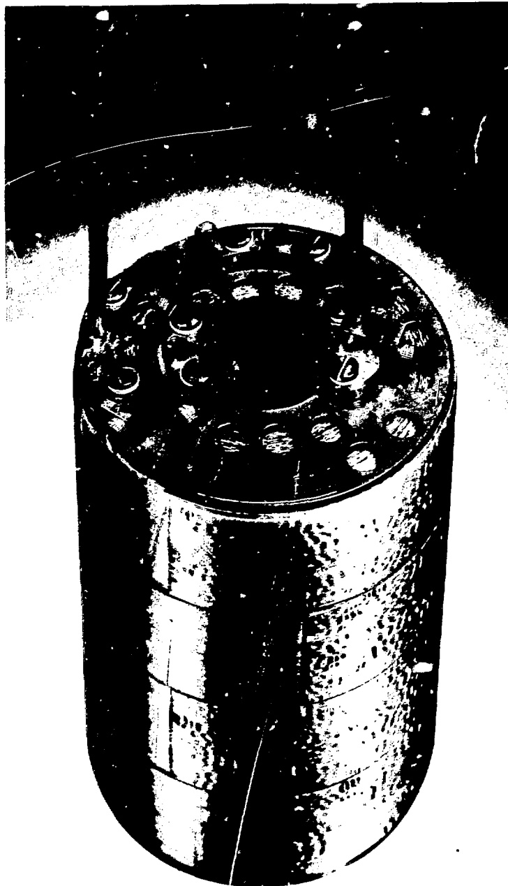
Figure 1. An early solenoid producing 112 kG.
