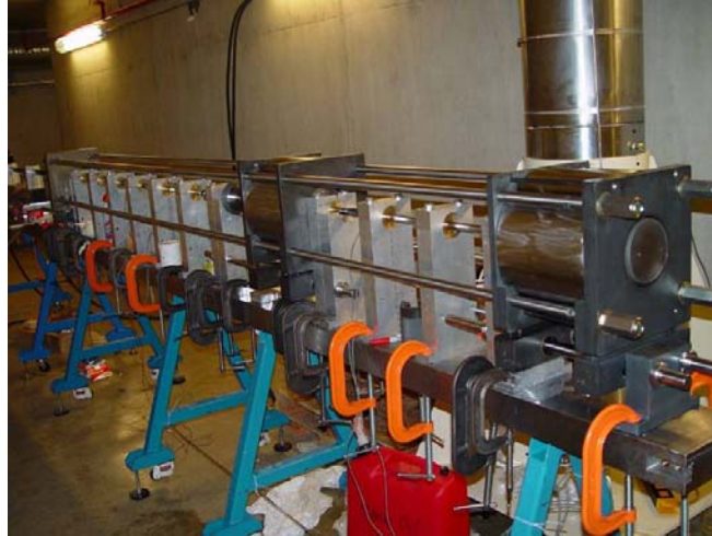
Figure 8. Photograph of the actual dynamic triaxial setup for sand experiments
