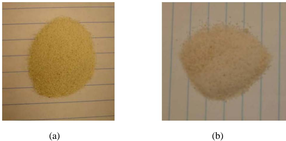
Figure 21. Sample leak check: a) Before applying pressure, and b) After applying 150 MPa confinement pressure
