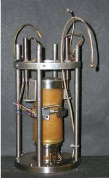
Figure 6. Photograph of the triaxial specimen assembly with instrumentation (Williams et al., 2006)
