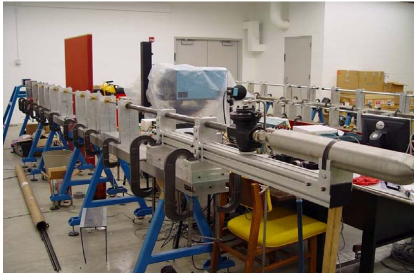
Figure 3. A photograph of the actual Kolsky bar for dynamic sand experiments
