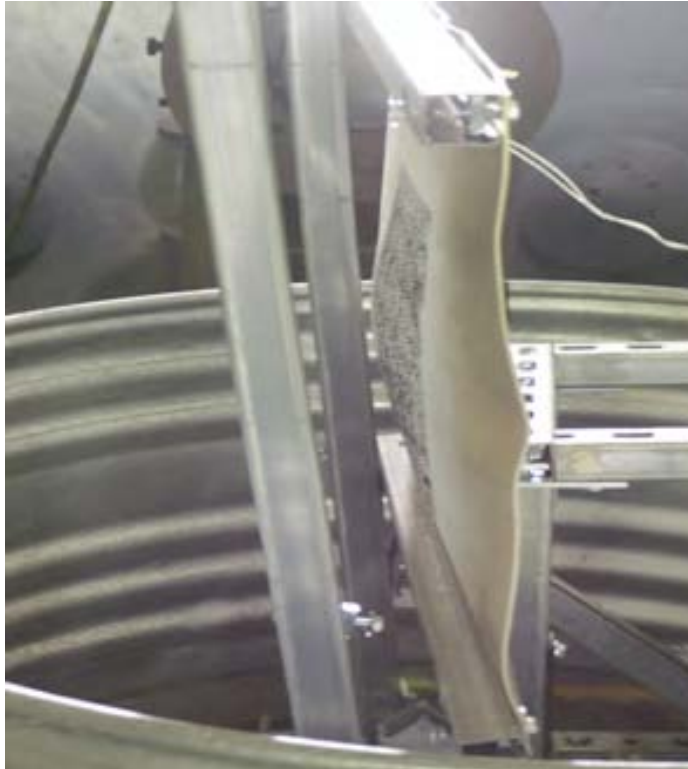
Fig. 6. Post-test, unmitigated, water-tamped plate deflection; note that aquarium is no longer present.
