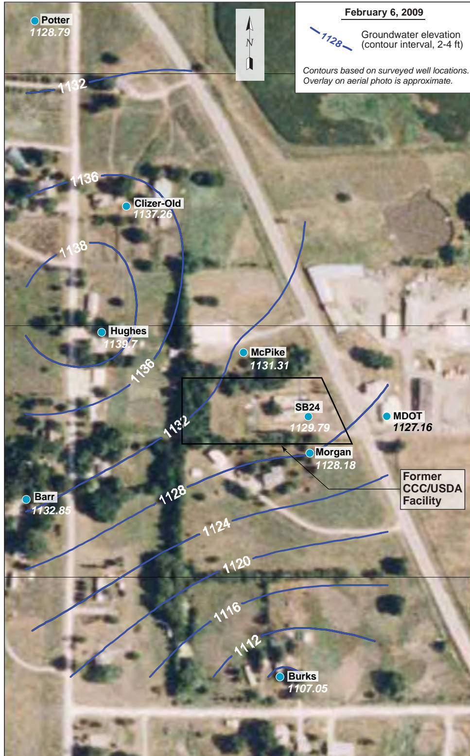
FIGURE 2.8 Water level contours constructed with data measured manually on February 6, 2009. The level for the Clizer “old” well is from continuously recorded data; the well was not accessible for manual measurement on this date. Source of photograph: NAIP (2007).
