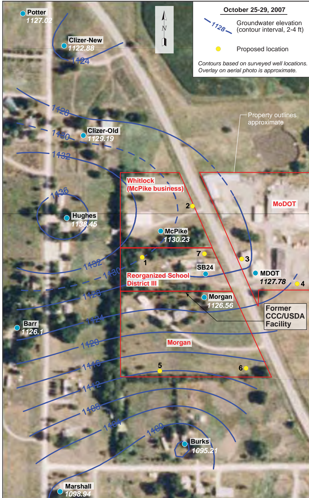
FIGURE 3.1 Water level contours based on groundwater levels measured on October 25-29, 2007, with proposed locations for the installation of shallow and deep monitoring well pairs during Phase II of the Savannah investigation. Source of photograph: NAIP (2007).
