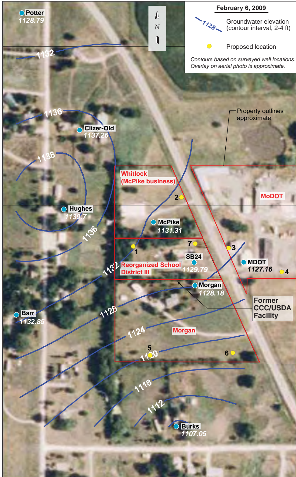
FIGURE 3.2 Water level contours based on groundwater levels measured on February 6, 2009, with proposed locations for the installation of shallow and deep monitoring well pairs during Phase II of the Savannah investigation. Source of photograph: NAIP (2007).
