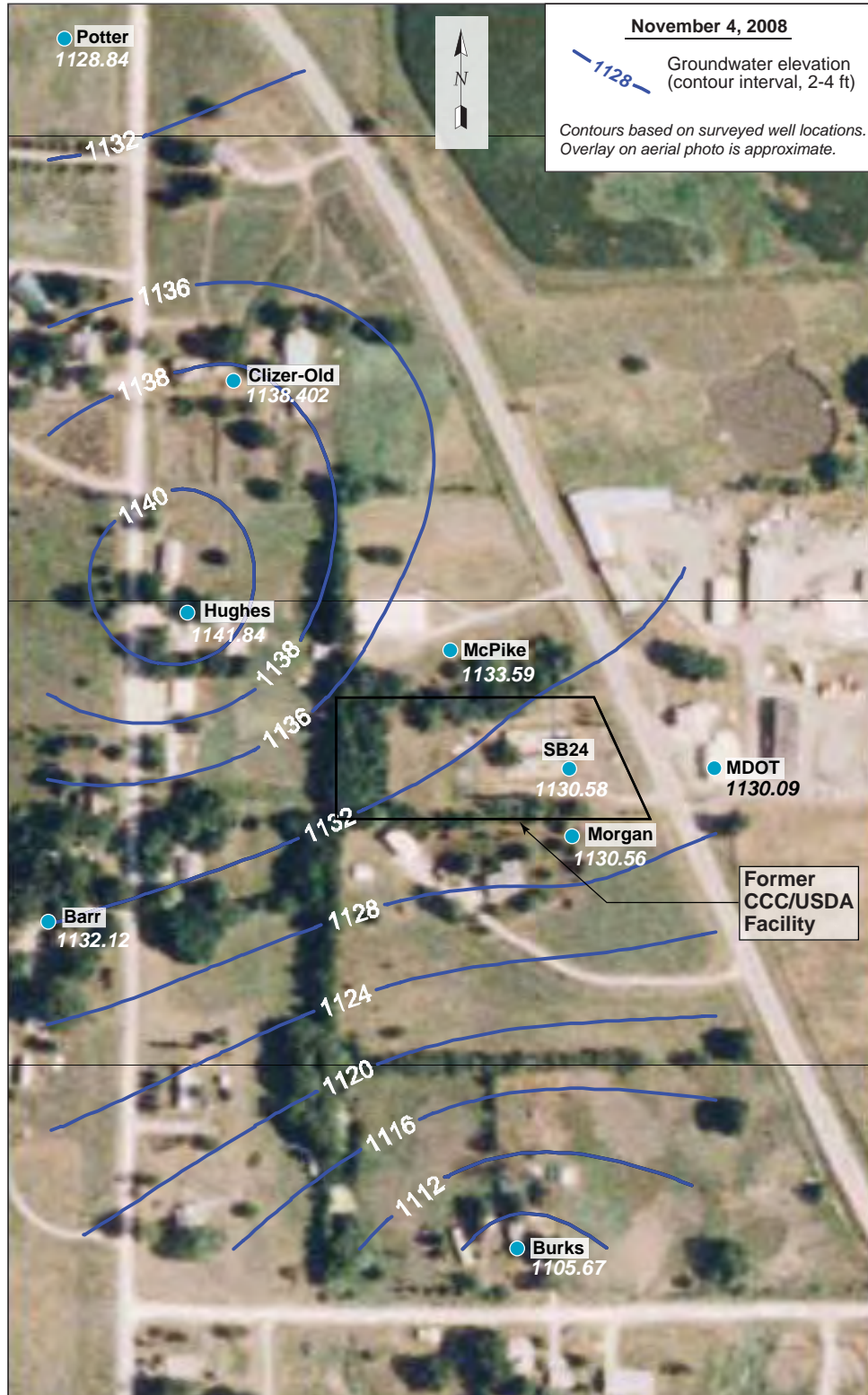
FIGURE 2.7 Water level contours constructed with data measured manually on November 4, 2008. The level for the Clizer “old” well is from continuously recorded data; the well was not accessible for manual measurement on this date. Source of photograph: NAIP (2007).
