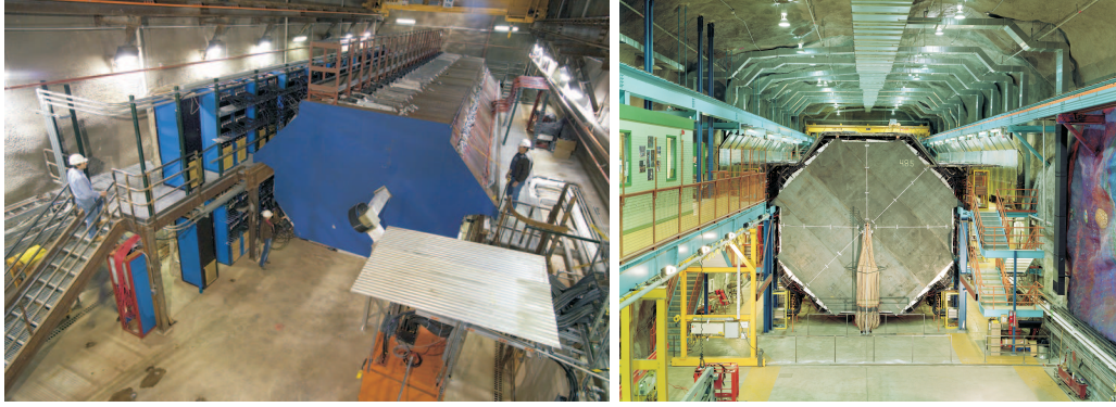
Figure 3.5: The MINOS near (left) and far (right) detectors.
