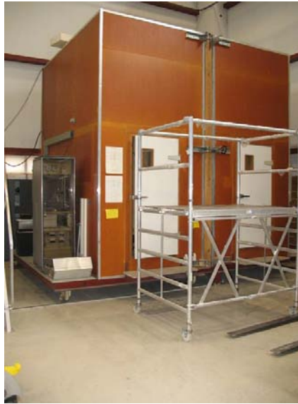
Figure 6 Photo of hot box. The cold chamber is to the right and the warm chamber is to the left. The metering area of the hot box is 2.45 \text{ m} \times 2.45 \text{ m} .
