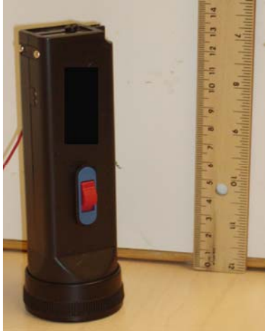
Figure 1-2. Flashlight A. Rechargeable 3 LED flashlight with a 1000 mAh rated battery.
