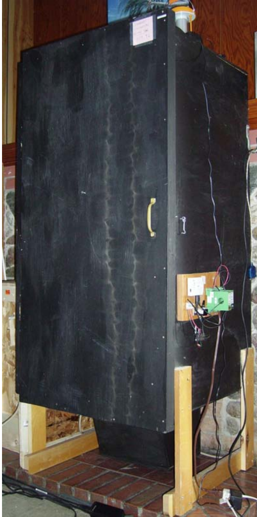
Figure 8. Dark Box used to perform the lamp discharge tests. Datalogging equipment on right-hand side of box.
