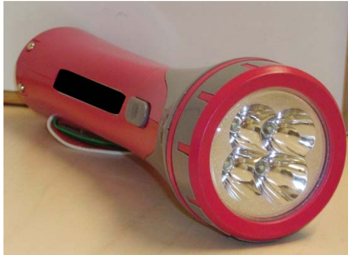
Figure 3-4. Flashlight B. Rechargeable 4 LED flashlight with a 800 mAh rated battery.
