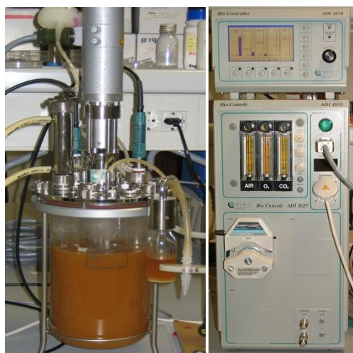
Figure 1.6. Biological reactors a) Biocontrol unit, Applikon Adi 1010 and console Applikon 1025; b) tank mechanically agitated (kindly loaned by “Laboratório de Engenharia e Biotecnologia Ambiental (LEBA)” from “Centro de Investigação Marinha e Ambiental (CIMA)” to realize the experiments.
