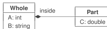
Figure 2: Example illustrating composition: the definition of one class of objects employing another class of objects in a part-whole relationship. In this particular example, an instance of a Whole class object must contain exactly one instance of a Part class object, and the label referring to the Part class object is inside . In XML, this symbol becomes the name of a subelement and the content of the subelement follows the definition of Part .
