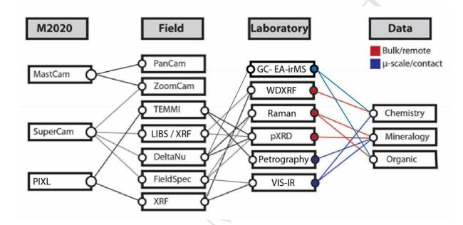
**Figure 1.** Schematic diagram showing the correlation between Mars 2020 (M2020) instruments, the CanMars M2020 stand-in field instruments (Field), and post-mission laboratory analyses used throughout this study. For definitions of laboratory collection methods, see Table 1. The far-right column indicates the type of laboratory data and scale appropriate to confirm in situ, insim science.
