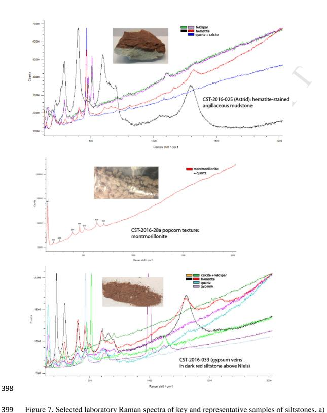
Figure 7. Selected laboratory Raman spectra of key and representative samples of siltstones. a)
