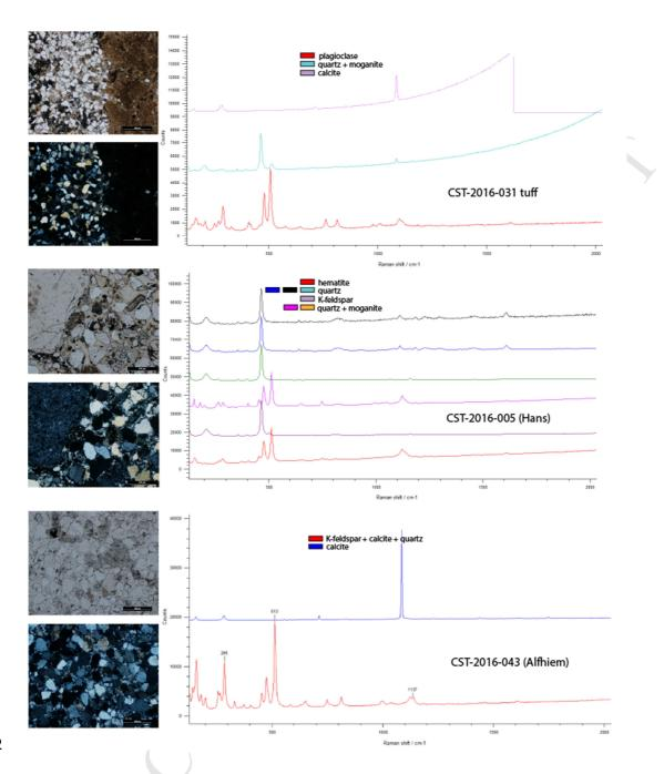
Figure 10. Selected laboratory Raman spectra of key and representative samples of tuffs and sandstones. Pictomicrographs are shown for context PPL (upper images) and XPL (lower images); all scale bars are 500µm. a) Tuff samples were dominated by plagioclase in Raman spectra, with quartz and moganite. The petrography shows altered glass and mineral grains (see Fig. 11 for detailed pictomicrograph descriptions). b) Hans sample, a younger silica cemented
