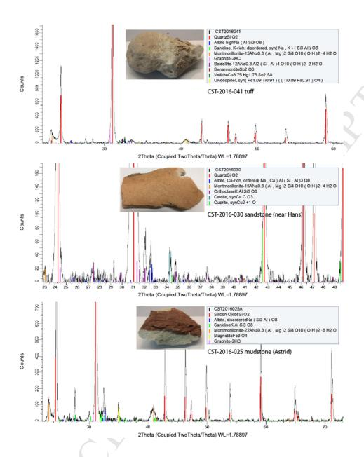
Fig. 9. Selected laboratory XRD patterns of key and representative samples of tuff, sandstone, and mudstone. Montmorillonite (with a strong low 2-theta 001 peak) and quartz (the tallest peaks, having the highest counts) are the dominant mineralogy signatures in all samples. The CST-2016-041 sample has mineralogy consistent with a tuff, including plagioclase and ulvospinel. Sample CST-2016-030 is a typical sandstone of the braided channel system in the
