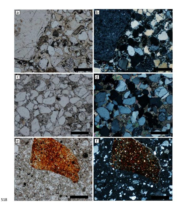
Figure 11. a and b) Thin section of CST-2016-005 (target Hans) in PPL (a) and XPL (b). All scale bars are  $500\mu m$ . Classified as subarkosic sandstone, clasts are  $100\text{-}400\,\mu m$  comprised of
