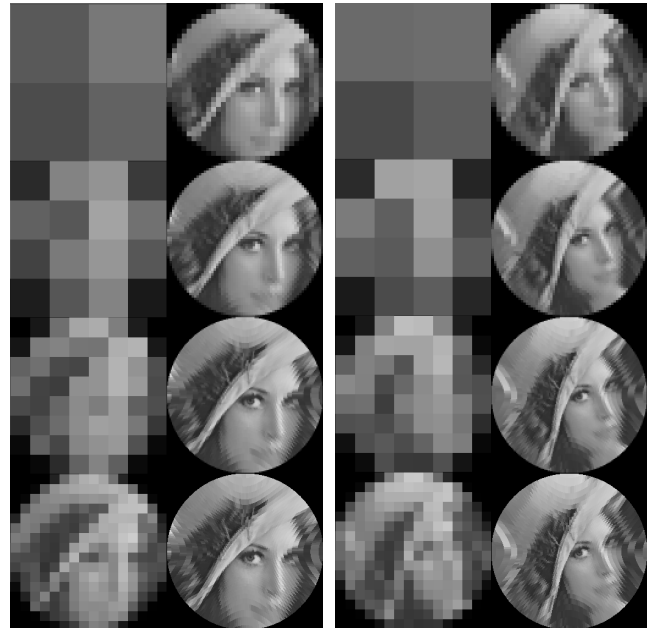
Fig.5 Multi-resolution images f_j, g_j by Haar wavelet
