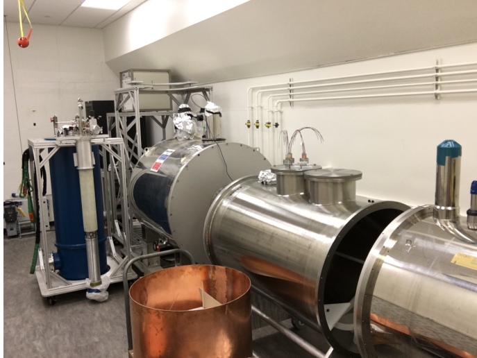
Figure 1: PTOLEMY prototype located in Jadwin Hall Physics Department, Princeton University (9 June 2017) showing the readout rack (far wall), Kelvinox MX400 dilution refrigerator (gas handler and pumps), 4.7 T Oxford Instruments 200/300 superconducting magnet, central vacuum tank (copper electrodes and HV feed-throughs) and 7.05 T Oxford Instruments 300/183 superconducting magnet.
