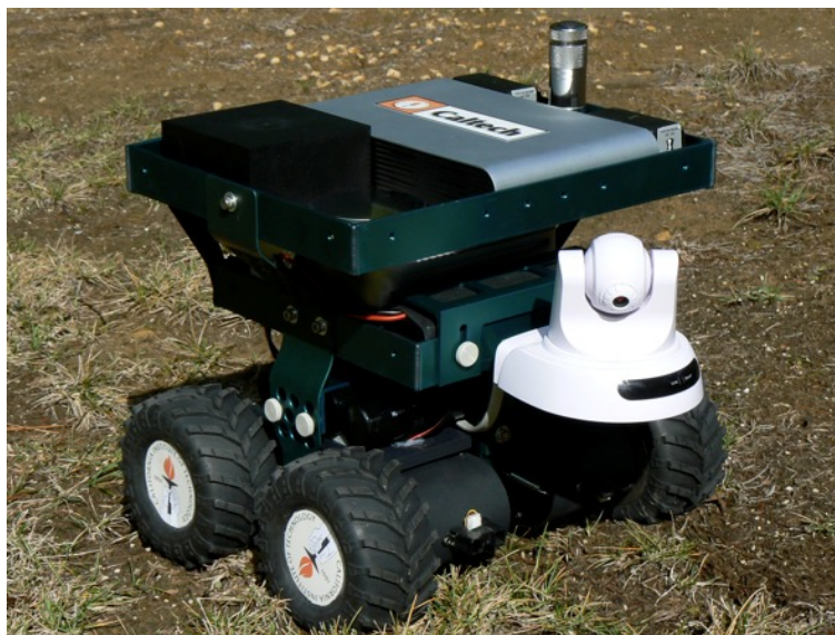
Fig. 3. Close-up of a ground-tier agent (i.e., rover), equipped with fully articulated, gimballed digital (science) camera (white), and a navigation camera beneath (from [13]).
