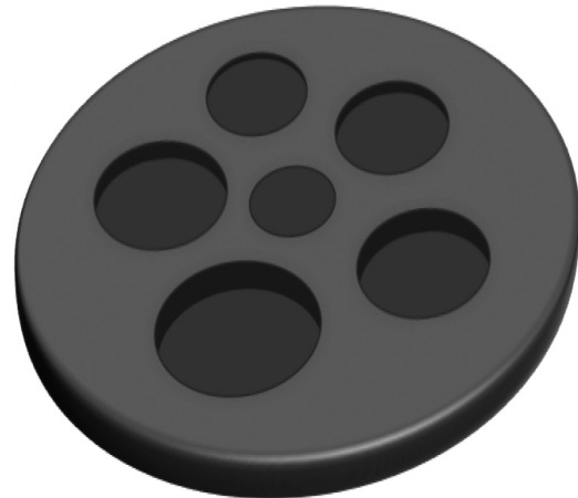
FIG. 1. Target design for the Ta baseplates used in this series. Each “pocket” cut in the baseplate creates a uniform step thickness. This allows six thicknesses to be studied per shot and improves uncertainties by correcting for reflections at the downrange surface. Reproduced with permission from Nguyen et al. , Phys. Rev. B 89 174109, 14 Copyright 2014 American Physical Society.
