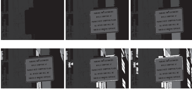
Fig. 5. Segmented potential backgrounds for various block sizes, k=64, 32, 16, 8, 4, 2 (left to right and top to bottom). Non-black regions are considered homogeneous. Each shade of gray corresponds to one region.
