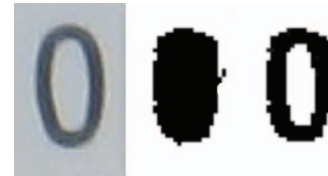
Fig. 7. (Left) Original image. (Middle) Text hole region. (Right) Text hole region after discarding pixels similar to surrounding background.
