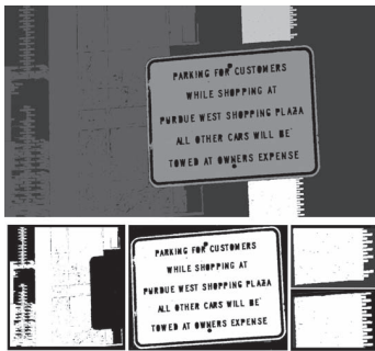
Fig. 6. Isolating the connected regions of an image: connected regions (top) and isolated regions of the image enclosed by exaggerated bounding boxes (bottom)
