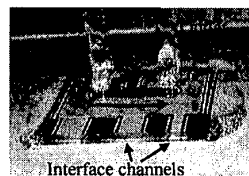
Figure 8: 1cm x 1cm glass interface die bonded to a glass substrate for initial testing
