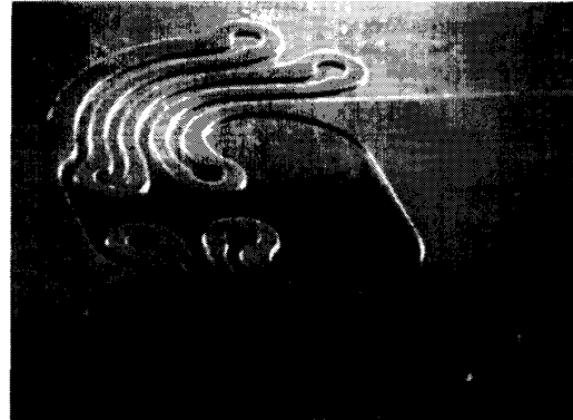
Fig. 3. SEM micrograph of a five-turn silicon microgimbal.
