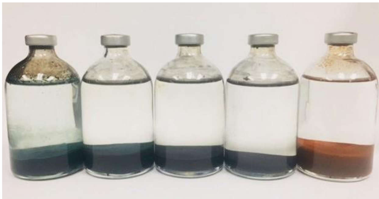
Figure S1: Iron hydroxide precipitates formed with different Fe(II):Fe(III) ratios. Left to right: 100% Fe(II), 75% Fe(II), 66% Fe(II), 50% Fe(II), 100% Fe(III).
