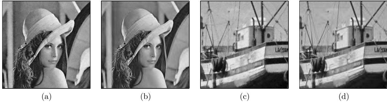
Figure 3. 256 \times 256 image recovery examples. Left: 'Lena' with K = 25000 . (a) Recovered from random projections via (12). (b) Optimal 6148-term wavelet approximation with same PSNR as (a). Right: 'Boats' with K = 20000 . (c) Recovered from random projections via (12). (d) Optimal 7207-term wavelet approximation with same PSNR as (c).
