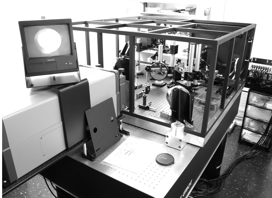
Fig. 6. Photograph of the coronagraph after initial alignment in the AMNH Astrophysics Lab's clean room. To the left is the Zygo interferometer used to simulate the AEOS beam to enable full testing in the lab prior to shipment to Maui. The residual wave front error through the entire system was 32 nm rms, 98.7% Strehl in the H-band. After shipping to Maui, the wave front error was measured at 29 nm. The alignment technique will be presented in a subsequent publication, currently in preparation. None of the optics moved, nor was any of the alignment work compromised during shipping.
