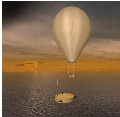
Figure 2-2. Examples of probes to send to Titan; a montgolfière balloon and a lake lander.
