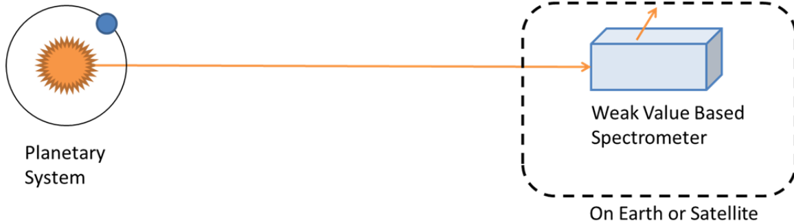
Figure IV-17 Light from a planetary system is used as an exo-planet detection probe. An exo-planet causes the light from the star to have a small periodic Doppler shift. A weak value based spectrometer [Starling2010b] can detect the presence of the exo-planet by observing the Doppler shift.
