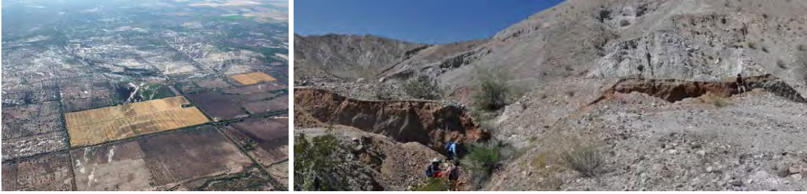
Figure 6. Left) Sand blows and liquefaction from the 2010 M 7.2 El Mayor – Cucapah earthquake. Right) fault scarp from the event (Fletcher et al, 2014).
