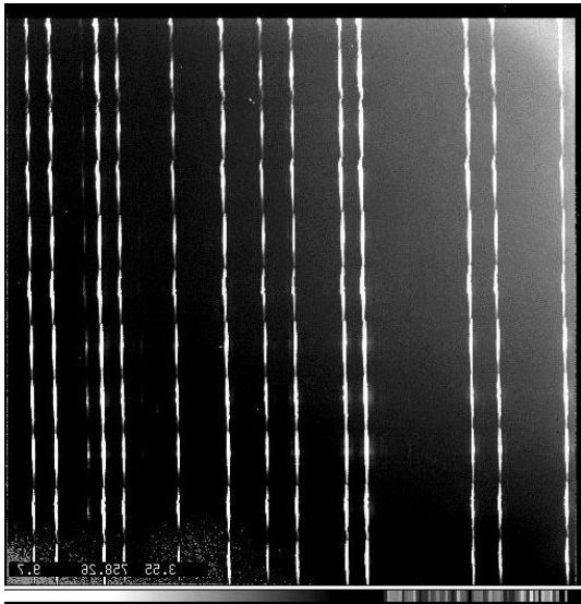
Fig. 19: Neon arc lines. Image of the fibers slit illuminated and diffracted by grating on the CCD.
