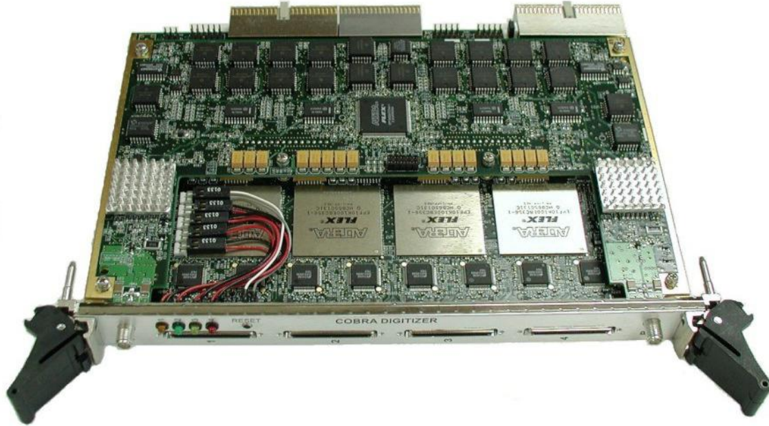
Figure 4. COBRA Digitizer Board; Two 1GHz 2-bit digitizers, 4 Altera FLEX10K FPGAs, a TI TMS320LC31 DSP, a PLX 9054 PCI interface, and LVDS front panel data distribution.
