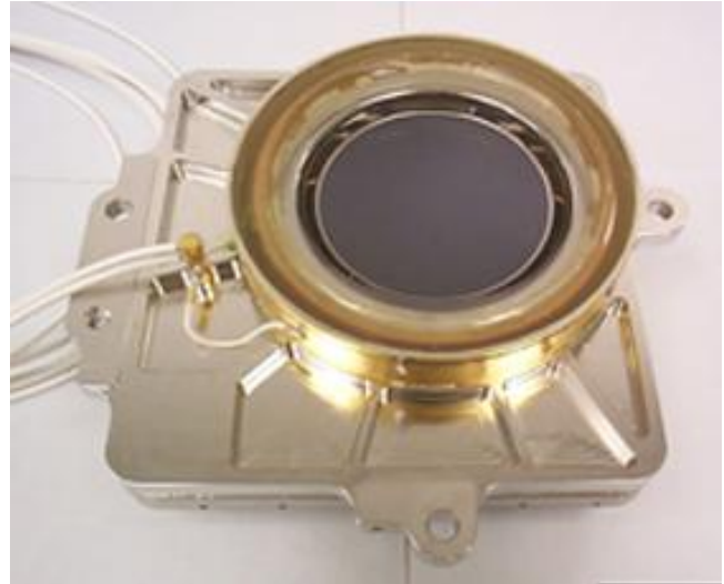
Figure 7 -- Flight NUV Detector
