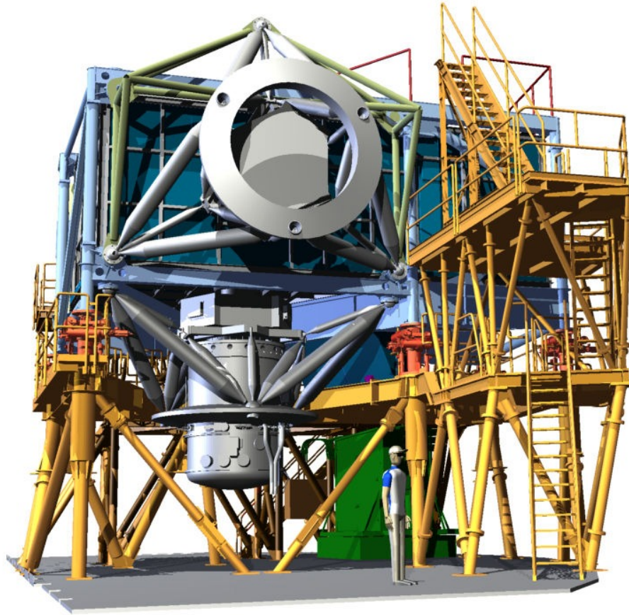
Figure 12: NFIRAOS on Nasmyth platform with IRIS underneath and NSEN on top
