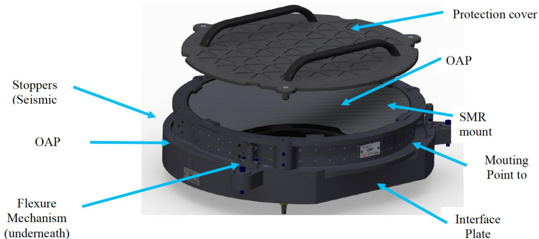
Figure 7: OAP mirror cell with interface plate
