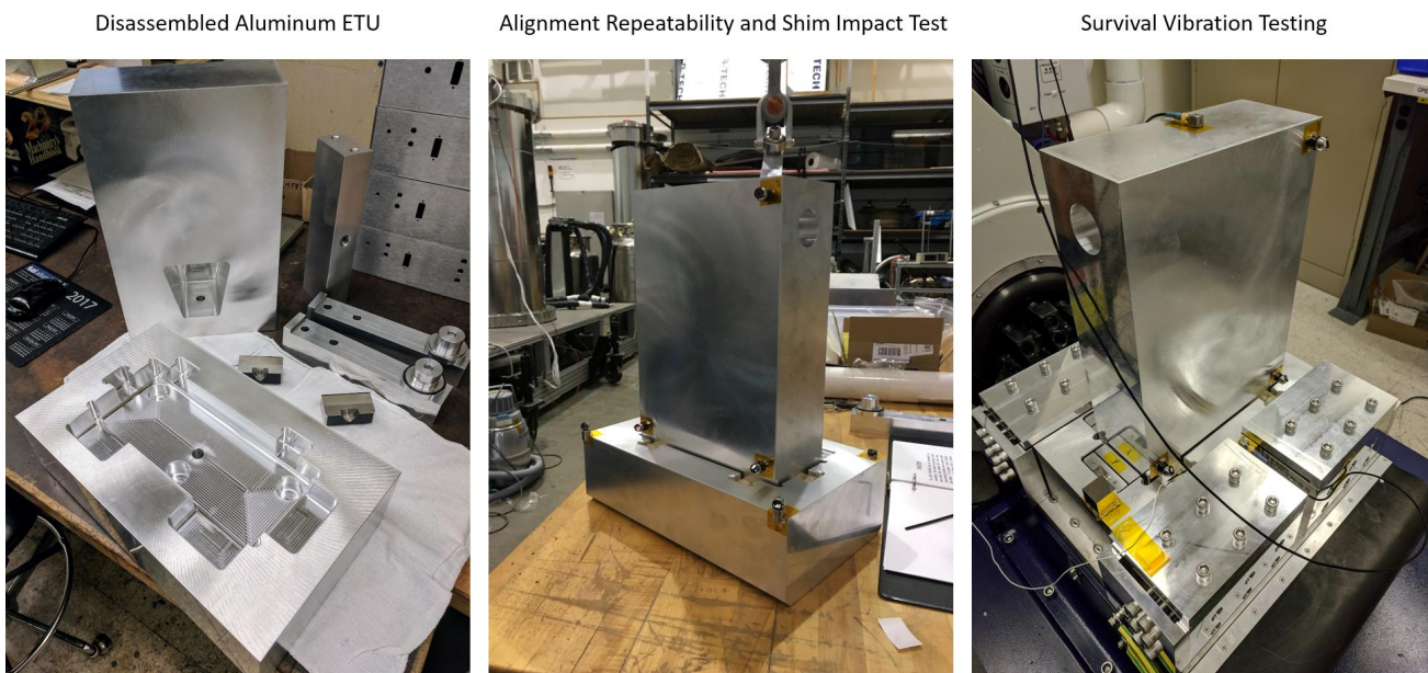
Figure 27. Disassembled aluminum ETU (left), ETU alignment repeatability and shim impact test configuration (center). Vibration test setup (right). Spherically mounted retro-reflectors were mounted to the aluminum ETU mirror and base to track relative alignment.
